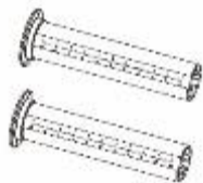
Ribbon Supply Spindle Ribbon Take-up Spindle
